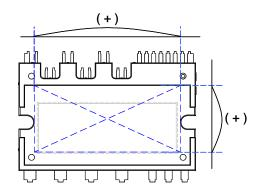
Figure 5. Flatness Measurement Position
