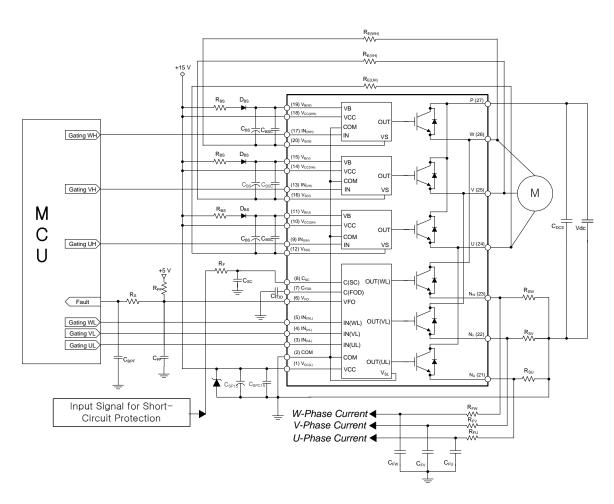
Figure 11. Typical Application Circuit
