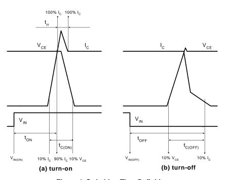
Figure 4. Switching Time Definition
