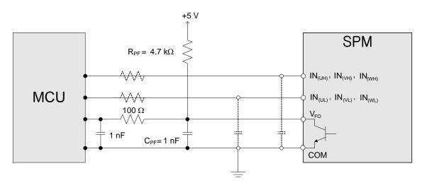
Figure 9. Recommended MCU I/O Interface Circuit
